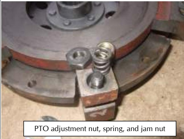
PTO adjustment nut, spring, and jam nut
